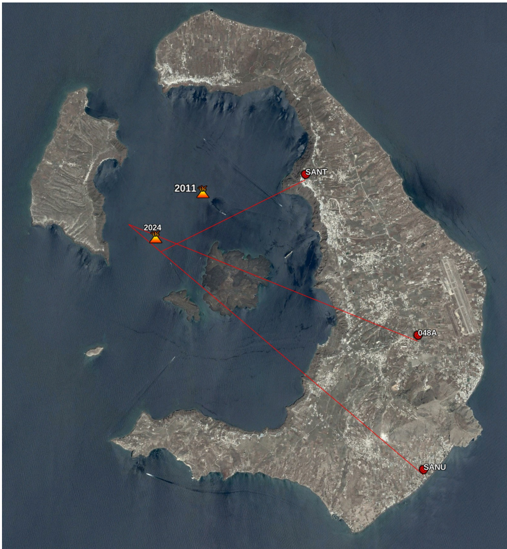
Figure 6. Triangulation of the centre of the inflation source using the azimuth of the deformation measured at the three stations SANT, 048A and SANU
